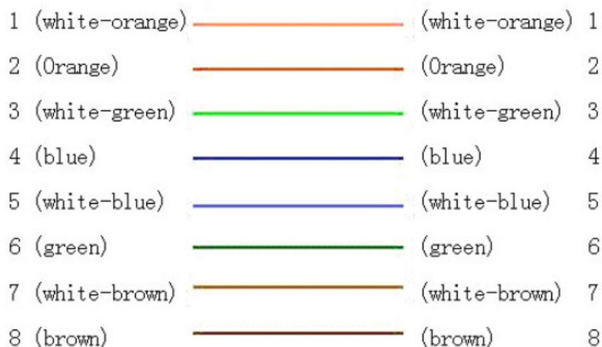
(2)UTP between the network port of camera and PC (Cross Cable):
