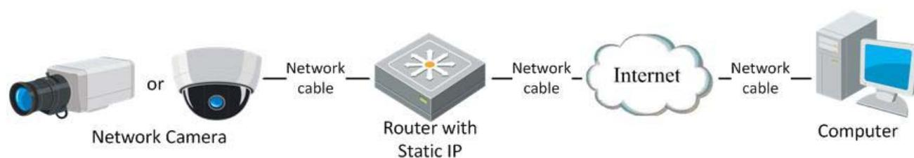
Fig. 3.1 Access IPC through Router with Static IP
