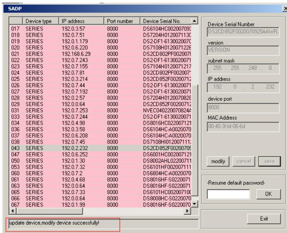
Input new IP address, subnet mask, and port number, and click “save” button. If a dialog pops up, showing “saved successfully”, that means you have modified the configuration information; if “saving failed” turns up, click the “cancel” button to quit it.
