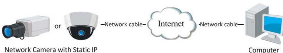
Fig.3. 2 Access IPC with Static IP directly
