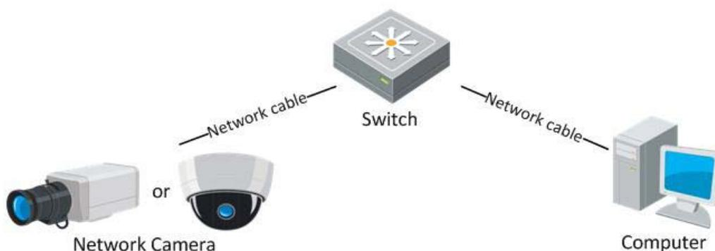
Fig. 1.2 Direct Line Connection
