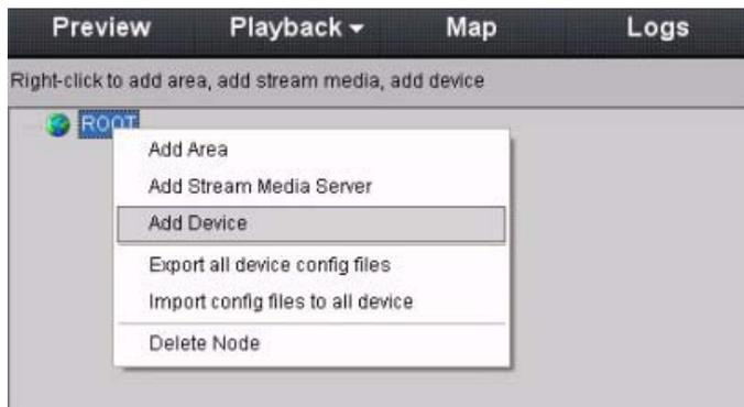
Input "Device Name" for your need. Select "Normal IP" from Register Mode. Input network camera's IP in *Device IP*, e.g. 192.0.0.64, *Port*: 8000, *User Name*: admin, *Password*: 12345. Select "TCP", "UTP", "MCAST" or "RTP" in [Protocol] for your need. Select "Main Stream" or "Sub Stream" in *Protocol* for your need. Finally, click *OK* to finish settings.
